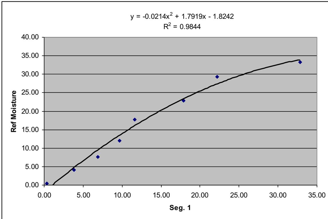
The coefficients displayed in the equation are the coefficients that should be entered into the sensors coefficients table, using the GPLP Reader software. Note that there will be a set of coefficients for *each* segment, take care to ensure that each segment is set to use the correct set of coefficients. The  $R^2$  value is a measure of how well the trend line fits the data (above 0.98 is good, the closer to 1, the better the fit is).
