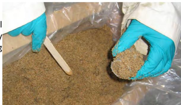
Cut away any excess soil from the open ends of the sampling ring, and also ensure that the outside of the sampling ring is free of soil.
