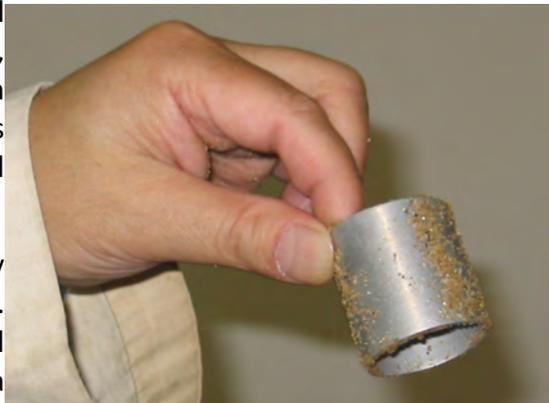
Calculate the volume of the sampling ring by measuring the interior diameter and cylinder length. The pictured example has length of 3.80 cm and interior diameter of 3.35 cm, corresponding to a volume of 33.5 cm<sup>3</sup> or 33.5 ml:
